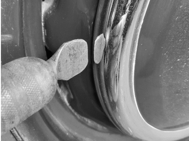
The shaped end of an official wheel brace slips into the gap between hubcap and wheel at one of the three flat areas.
